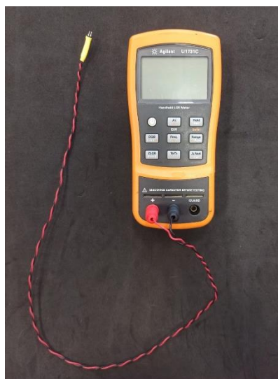
Figure 1. Digital LCR meter coupled with the metallic probe.
