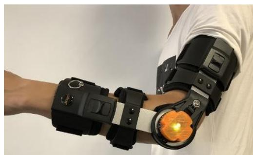
Figura 3: OREHAB-ARM Smart Brace.
