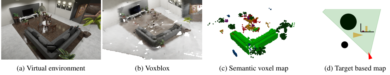
Figure 3: Different state representations for the problem of active perception. For the environment shown in 3a, the Voxblox map in 3b is used to store occupancy information for geometric active perception, the semantic voxel map in 3c is used for active semantic mapping. In other cases, a simpler target-based representation with information about the target position and class, and other environment information like occluder positions might be enough as shown in 3d.
