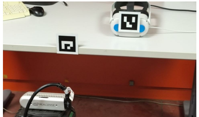
Figure 7: Setup to measure accuracy in position and rotation error.
