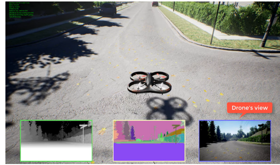
Figure 1: AirSim simulation of an UAV equipped with sensors.
