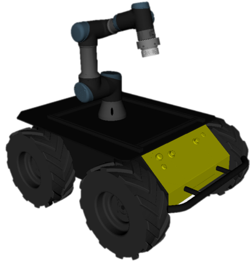
Figure 3: UR3 mounted on Husky mobile robot
