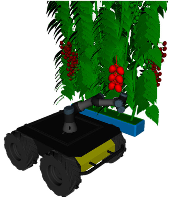
Figure 5: Husky, ur3 and plant simulation
