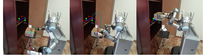
Figure 5: Dual-arm pick-and-place task with ADAM. (Left) Approach and grasp, highlighting initial frames ( T_{obj}^L, T_{obj}^R ) and updated 6D shelf goals ( T_{shelf}^L, T_{shelf}^R ). (Middle) Coordinated transport via zero-shot adapted trajectories (purple/teal) seamlessly connecting start and goal poses while maintaining the closed kinematic chain. (Right) High-precision placement at novel configurations, proving robust generalization from a single demonstration.
