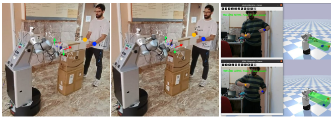
Figure 6: Human-robot transport with ADAM. (Left and Middle) Real-world execution. The visual tracking system monitors the human operator's hands ( T_{hum}^L, T_{hum}^R , marked with blue and orange dots) to continuously compute the via-points for the robot's end-effectors ( T_{obj}^L, T_{obj}^R ), preserving the closed kinematic chain. (Right) Real-time example using ADAMSim.
