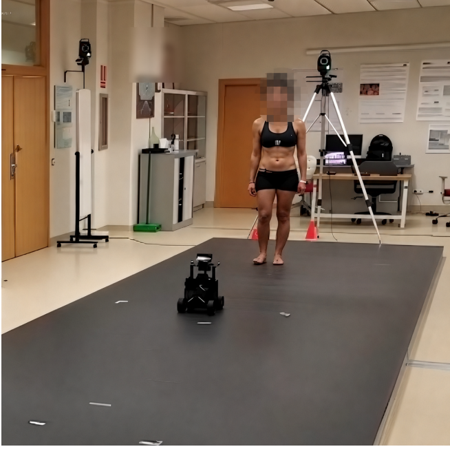
Figure 2: Experimental setup used for gait acquisition with the robot-assisted RGB-D system and the VICON reference motion-capture system.
