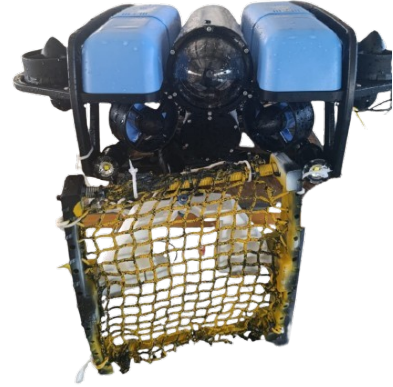
Figure 2: BlueROV2 heavy platform with integrated patching end-effector.
