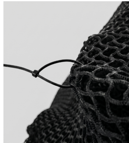
Figure 13: Zip-tie ready to be tightened.
