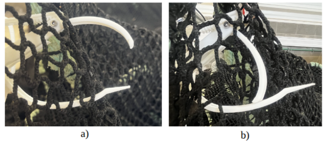
Figure 9: a) Tool's head reaching the net rupture (posStart), b) the upper jaw closes at a predefined position (pos1).
