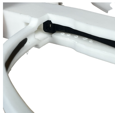
Figure 10: Zip-ties reaching the mechanical stop.
